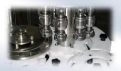
Mechanical pincers made from stainless steel, the three sector mechanical pincers is for closing special threaded caps or special applications, which can be installed on the magnetic torque head.
