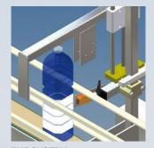
THE SYSTEM Ideal to ensure the presence of wraparround or sleeve labels, opaque or partially transparent, applied on any type of container.
